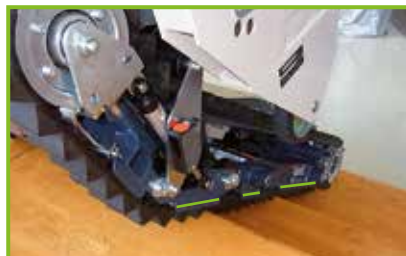
Easy and safe landing by flexible frame
